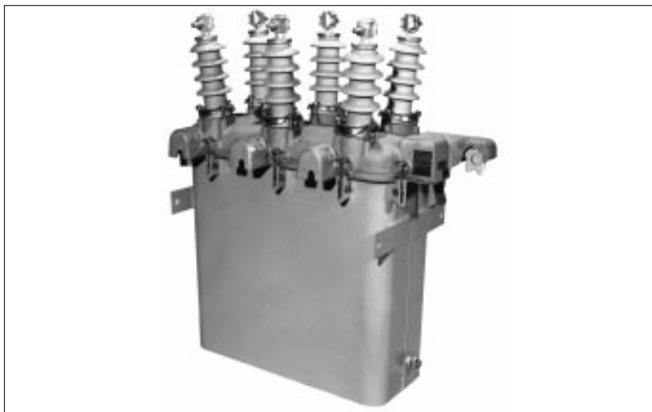
Figure 2. Type 6H recloser provides single-phase tripping and three-phase lockout.
